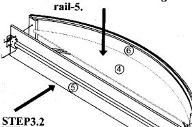
Push to make curve rails-6 and staight rail-5 close by each end sides and align the hole before using bolt to tighten.
